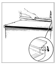
When drawers and covers are back in place, reinstall the gasket at the rear of the Sealed & Fresh drawer. Fit the end of the plastic drawer support into the sloton the gasket, with the rubber gasket flap facing you. Make sure the gasket snaps into place.
